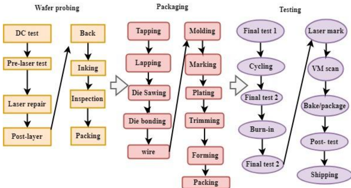
Figure 5.1 Process Flow in Semiconductor Packaging
