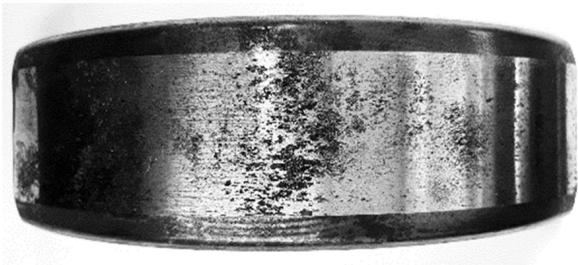
Fig 1.3(b): Material-fatigue based failure of a bearing
