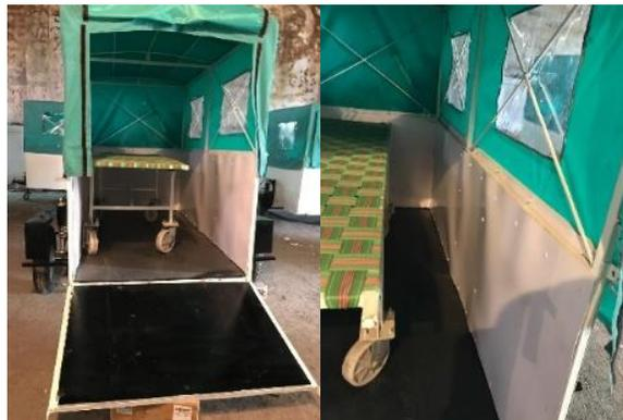
*Figure XV – Gate and Ramp Mechanism*
