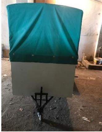
*Figure IX – Grambulance Showing the Hitch setup*
