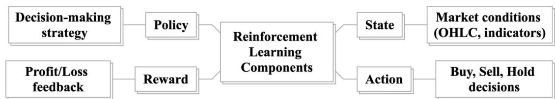
Figure 5:Fundamental Concepts of Reinforcement Learning
